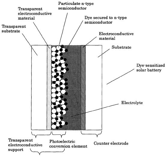
Electrode comprised of photoelectric conversion element
